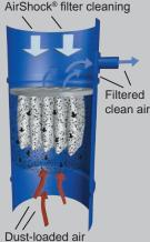
The AirShock® inflates the filter pockets instantaneously. Accumulated dust drops off and falls down into the collection container.
