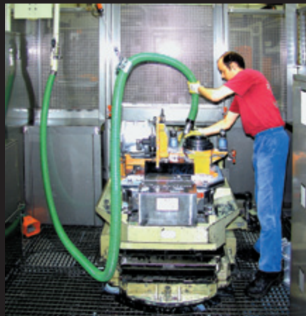
Cleaning of production machines in the metal working industry. Extraction of swarf and coolant.
