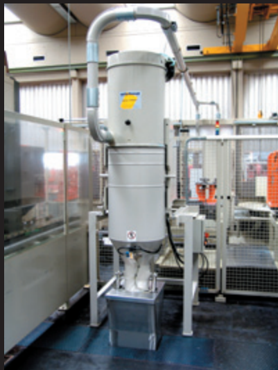
At maximum filling level the TowerVac discharges into an underfloor conveyor. The suction hose is connected to a pipe work system.
