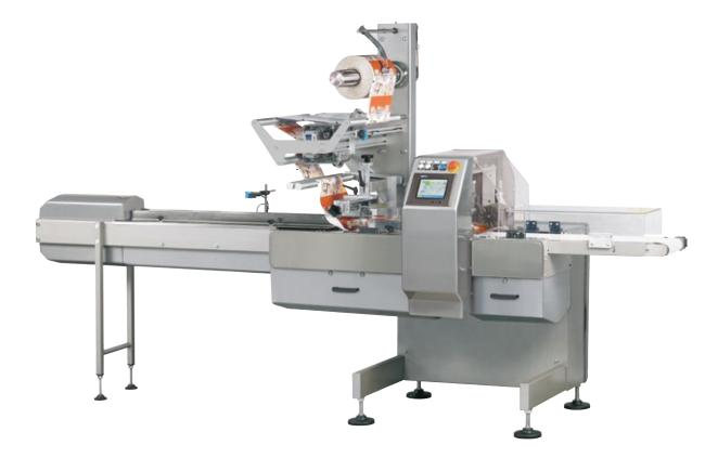
This automatic **ASCO** Wrapping Machine APM50 is specially designed for the use of dry ice slices and / or blocks. All parts in contact with the product are made of stainless steel. Automatic pitch change on conveyor and all motors are torque controlled. The temperature for welding is shown on the display and is electronically controlled. The control panel consists of various instruments and visual alarms and is equipped with a self-diagnostic device.
