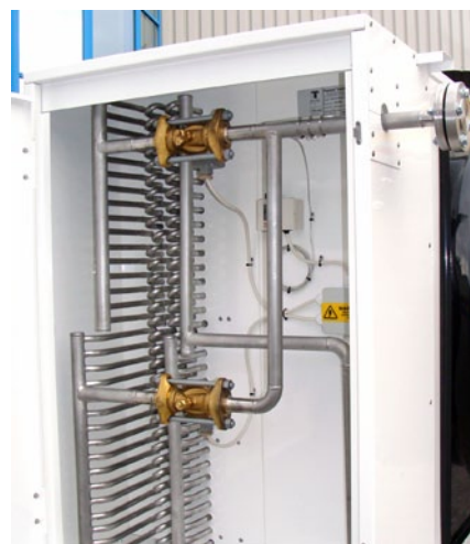
1'000 kg/hr Atmospheric CO 2 Vaporiser Two independent coils
