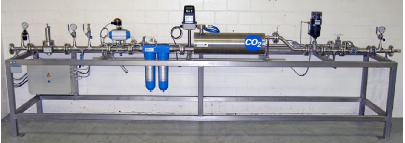
ASCO CO 2 Dosing System (single line)
